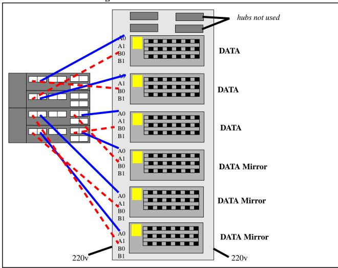
Note: Each adapter is on a separate sbus. Each mirrored pair uses separate adapters on separate system boards. Don't use the array hubs or power sequencer.
