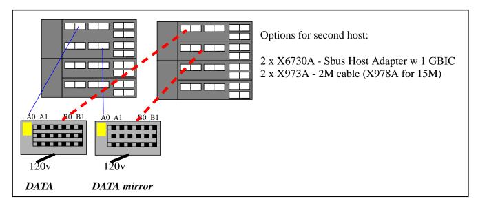
Note: The second host would connect to the B0 array ports. This gives better fault tolerance and performance as data traffic or errors on one host's loop will not effect the other host.
