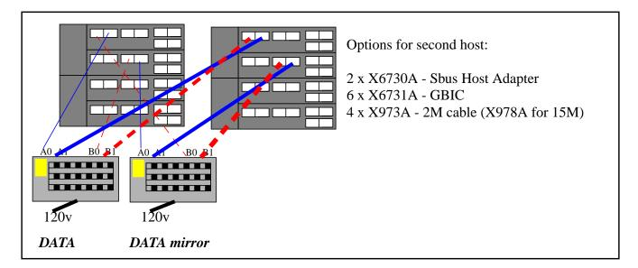
Note: For hosts that use an array disk for booting you should configure one host to boot to loop A, the other host to boot to loop B. This will prevent data traffic or errors from one host effecting the other.
