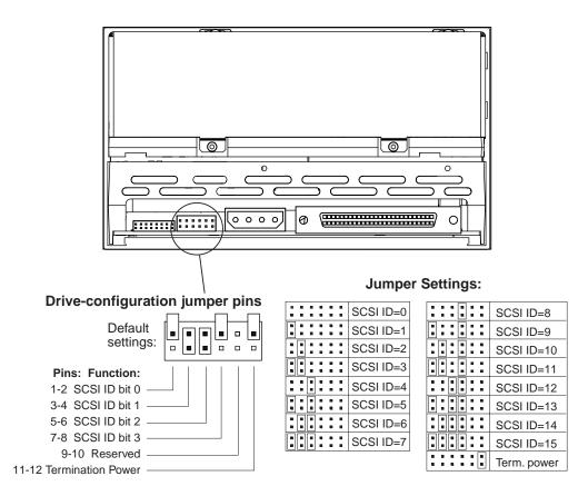
Figure 3. Back view of the Viper 200 internal drive, showing jumper settings
