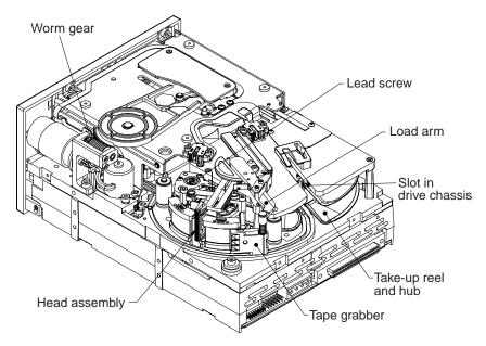
Figure 13. Diagram of Viper 200 showing key components used in manual cartridge tape removal (no tape cartridge in drive).
