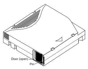
Figure 19. LTO cartridge with door open to show leader pin.
