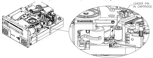
Figure 11. Diagram of Viper 200 showing leader pin inside LTO cartridge (tape *not* threaded on take-up hub)
