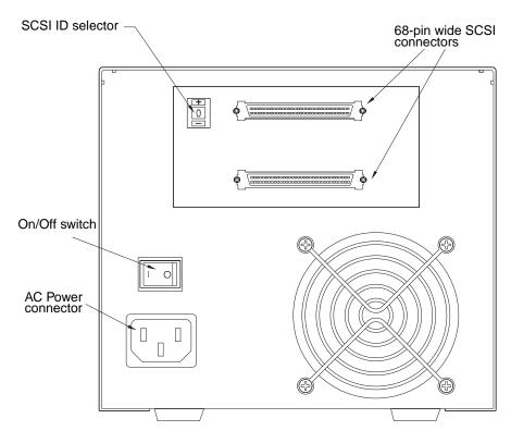
Figure 7. Back of external Viper 200 showing switches and connectors
