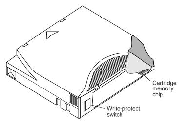
Figure 20. LTO cartridge showing cartridge memory and write-protect switch
