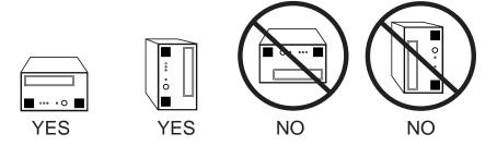
Figure 4. Acceptable mounting orientations for internal Viper 200.
