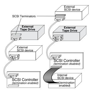
Example 1: SCSI termination in a system that has only external SCSI devices.
