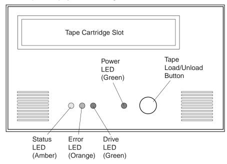
Figure 9. Generic front panel display for Viper 200
