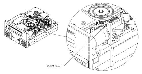
Figure 17. Diagram of Viper 200 showing worm gear
