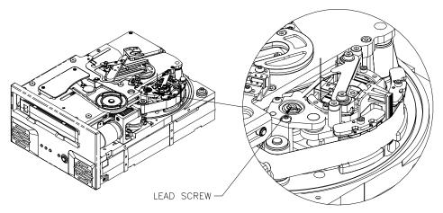
Figure 14. Diagram of Viper 200 showing lead screw (tape threaded on take-up reel)
