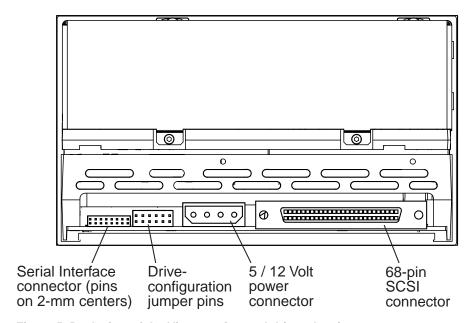
Figure 5. Back view of the Viper 200 internal drive, showing connectors
