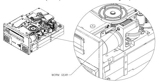
Figure 12. Diagram of Viper 200 showing worm gear
