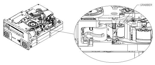
Figure 16. Diagram of underside of Viper 200 showing tape grabber near cartrdige
