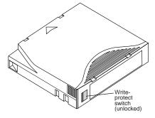
Figure 10. Ultrium cartridge showing write-protect switch
