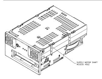
Figure 15. Diagram of underside of Viper 200 showing supply motor access hole
