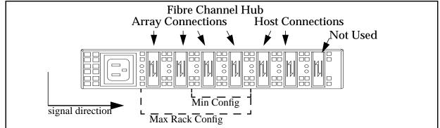
The factory installed hub cable configurations increases signal margins between the arrays and the hosts. The signal direction is left to right and its best to minimize the loop distance for data sent from the array. Hub slot 6 is not used. Slots 4 and 5 are for host connections starting with 4. Slots 0 through 3 are for arrays starting with 3.
