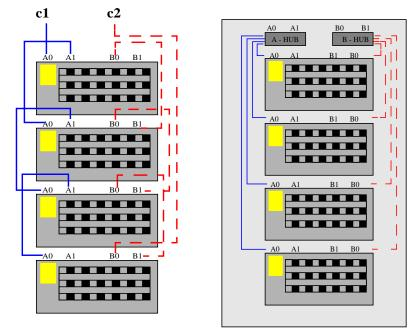
Multiple arrays can connected to the same host connect/s and fc-al loop/s using daisy chained cables or hubs. The functionality and performance is identical but hubs are generally prefered for the cabling simplicity and higher fault tolerance.
