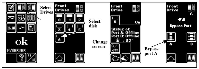
**Note** – Component bypasses are not preserved after a reset or power on. Default state after power on is all components enabled.
