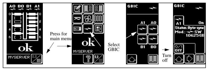
To loop back through the IB, bypass the IB/loop port for both backplanes.
