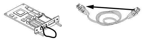
Or loop back connector plugs can be purchased from fibre cable suppliers. Below is one vendor source:
