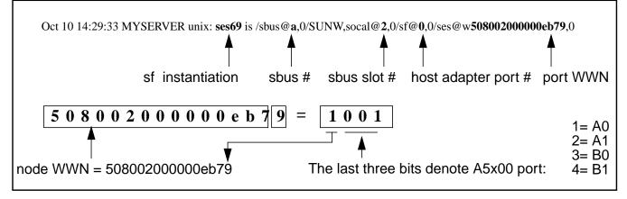
**Note** – The array path uses a unique world wide numbers (WWN) to identify the array. The WWN is stored on the interconnect assembly. You must use the luxadm remove\_device and insert\_device commands when replacing the interconnect assebly to rebuild the ses device paths.
