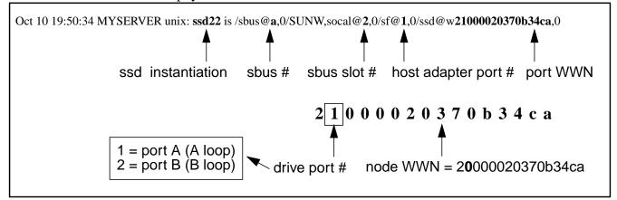
**Note** – The disk addresses use unique world wide numbers (WWN). You must use the luxadm remove\_device and insert\_device commands when replacing disks to rebuild the device path.
