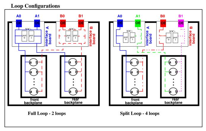
The A5x00 arrays can be configured to run as either 2 or 4 fc-al loops.
