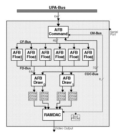
Figure 4. Sun Elite3D m6 graphics chip-level diagram
