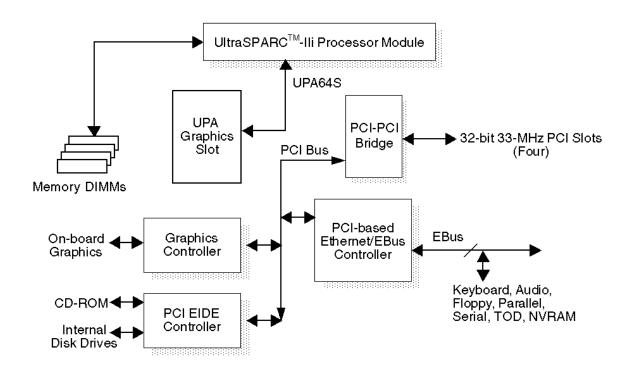
Figure 2. Sun Ultra™ 10 workstation block diagram
