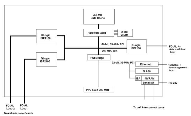
Figure 4. Controller architecture
