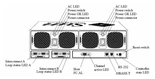
Figure 6. Rear view of the Sun StorEdge T3 controller unit
