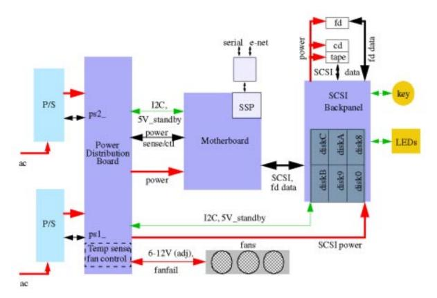
Figure 3: System architecture of the Sun Enterprise™ 250 server
