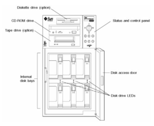
Figure 4: Front view of Sun Enterprise 250 server, disk access doors open
