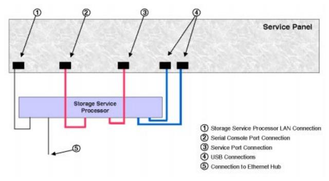
Figure 5. Storage Service Processor without Sun StorEdge Remote Response
