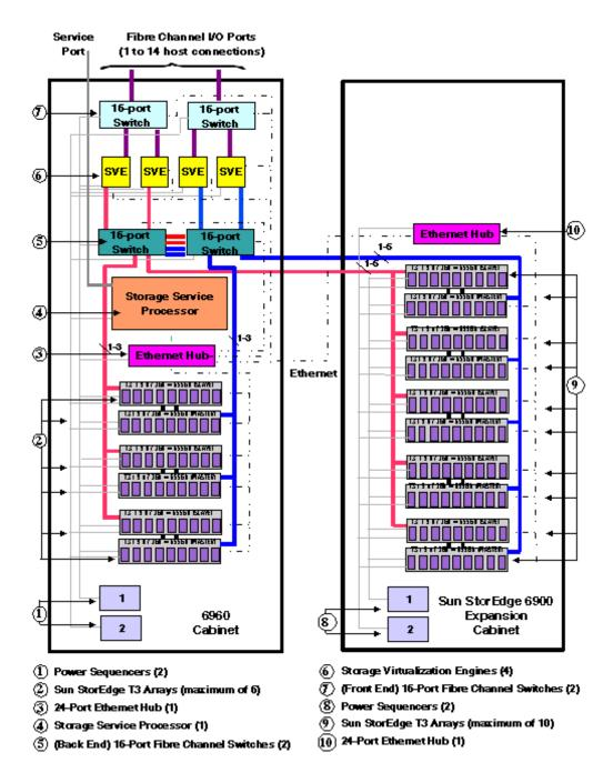
Figure 4. Sun StorEdge 6960 system cabinet configuration
