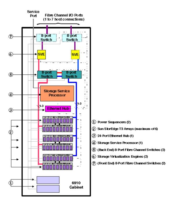
Figure 3. Sun StorEdge 6910 system cabinet configuration
